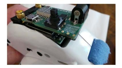
Keep pushing gently until you are able to slide the connector pins inside the relevant slot. There's no way to misplace pins, just be sure that pins enters correctly. Push down the module to place it completely in position. First time maybe it requires more time but you'll get used in short, it's not difficult
