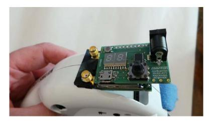
Gently slide the module SMA connectors inside the clip pushing towards the middle of the googles
